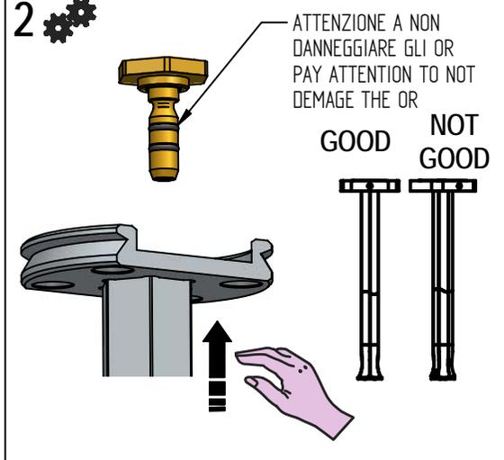
**SOSTITUZIONE AERATORE / AERATOR REPLACEMENT**
